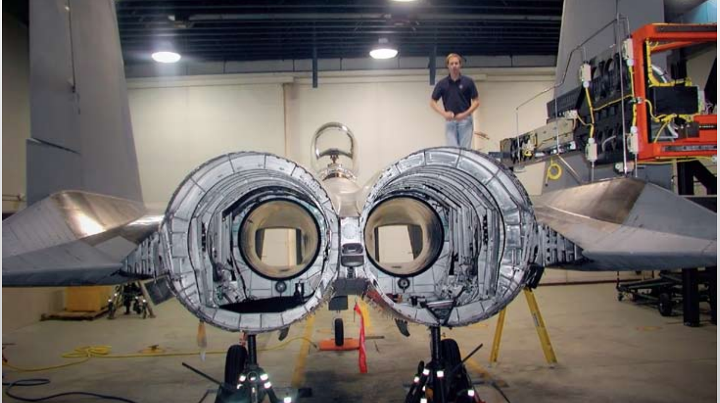
The Air Force's new multi-axis X-ray is used here to detect aging aircraft problems like foreign object damage, corrosion and internal moisture on an F-15 Eagle at the Warner Robins Air Logistics Center at Robins Air Force Base, Ga. The system is projected to save the Air Force time and money, increase worker safety and reduce environmental hazards.
