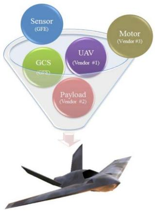
Figure 9: SUAS Modularization from Multiple Sources
