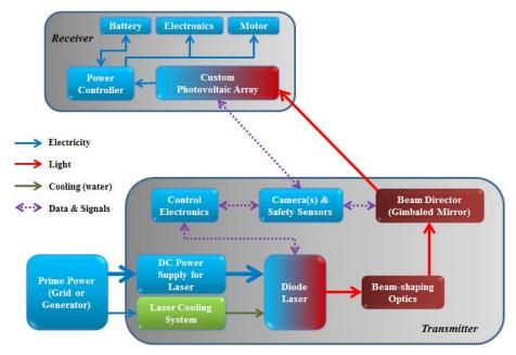
Figure 11: LaserMotive's Wireless Extension Cord<sup>40</sup>
