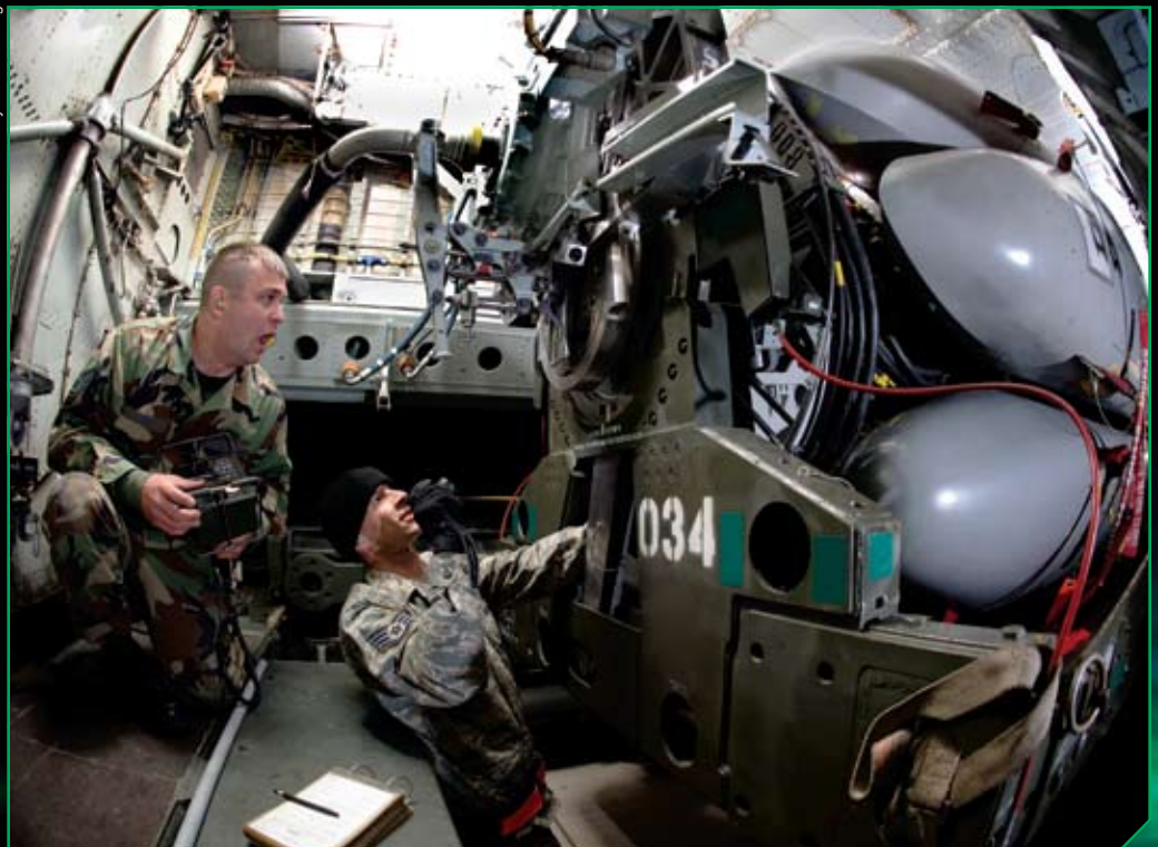
Staff Sgts. James Pavatt (right) and Jon Tokay use a munitions handling unit to raise a fully loaded rotary launcher carrying eight AGM-86B/C air launched cruise missiles to the on-board assembly inside a B-52 Stratofortress at Barksdale Air Force Base, La.
