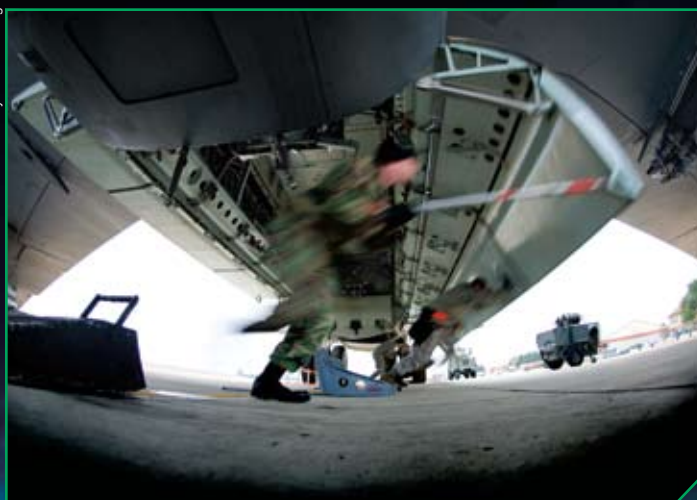
Senior Airman Matthew Paul Rivera and his team must work together to manually lift one of the 800-pound B-52 Stratofortress' bomb bay doors at Barksdale Air Force Base, La. Once locked into position, a rotary launcher can fit under the bomber.
