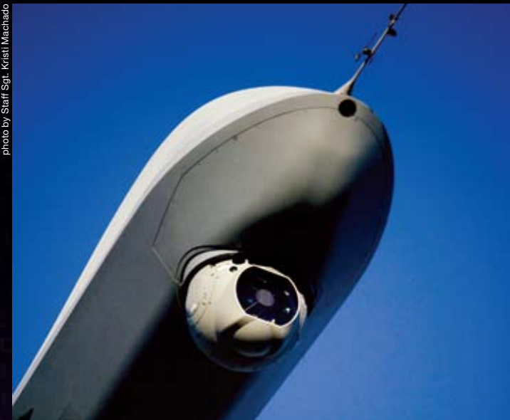
The MQ-9 Reaper uses a multi-spectral assembly during a mission. The assembly provides infrared sensor capability, color/monochrome daylight video and image-intensified video.
