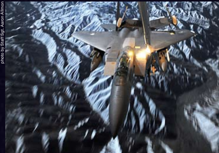
A KC-10 Extender from the 908th Expeditionary Aerial Refueling Squadron refuels an F-15E Strike Eagle from the 391st Expeditionary Fighter Squadron. The F-15E extends ISR capability with nontraditional sensing using the Sniper pod mounted under its left intake.
