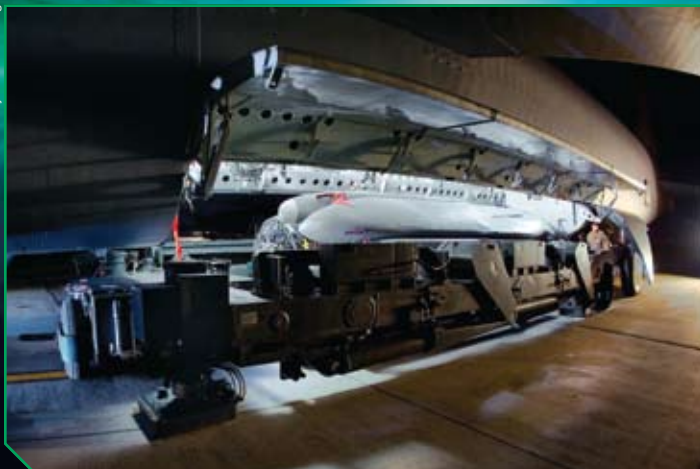
Under a B-52 Stratofortress at Barksdale Air Force Base, La., Airmen maneuver an 80,000 pound munitions trailer carrying eight AGM-86B/C air launched cruise missiles.
