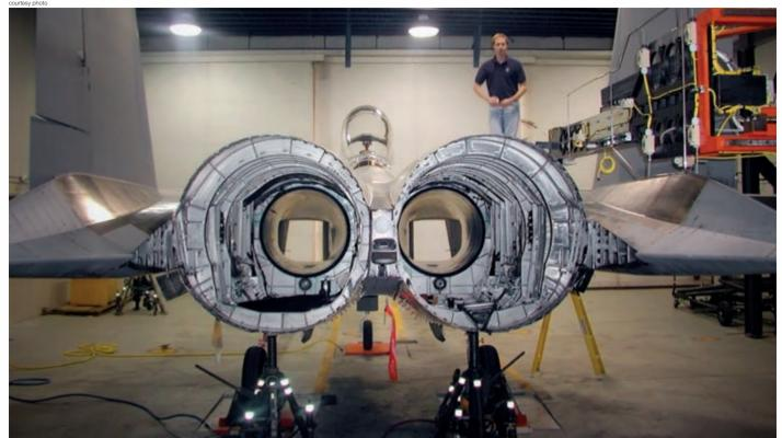
ROBINS AIR FORCE BASE, Ga. -- The new multiaxis X-ray detects aging aircraft problems like foreign object damage, corrosion and internal moisture on an F-15 Eagle at Warner Robins Air Logistics Center here. The system is projected to save the Air Force time and money, increase worker safety and reduce environmental hazards.
