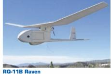
Primary function: Provides day/night reconnaissance and surveillance with low altitude operation. Speed: 20-40 mph. Dimensions: Wingspan 4 feet 5 inches. Endurance: 60-90 minutes. Operating altitude: 100-500 feet.
