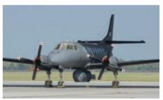
Primary function: Counterdrug. Speed: 288 mph. Dimensions: Wingspan 57 ft.; length 59 ft. 4 in.; width 16 ft. 8 in. Range: 1,380 miles. Crew: Two.
