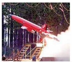
**BQM-167 Subscale Aerial Target** Primary function: Aerial target. Speed: 691.2 mph. Dimensions: Wingspan: 11 ft.; length 20 ft.; height: 4 ft. Crew: None.
